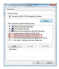
**5.** Click the "Use the following IP address" option in the **General** tab in the **Local Area Connections Properties** window and enter the desired IP address in the space offered. Then click the "Use the following DNS server adresses" option on the same tab and enter the desired DNS server information.
