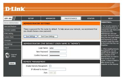
IP Allowed to The Internet IP address of the computer that has access to the Broadband Router. If you input an asterisk (\*) into this field, then any Access: computer will be able to access the Router. Putting an asterisk (\*) into this field would present a security risk and is not recommended.
