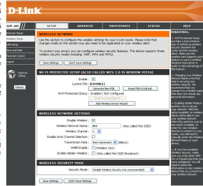
Transmission Use the drop-down menu to select the appropriate Transmission Rate in Mbits per second. Many users will want to use the default setting. Rate: Best (automatic).
