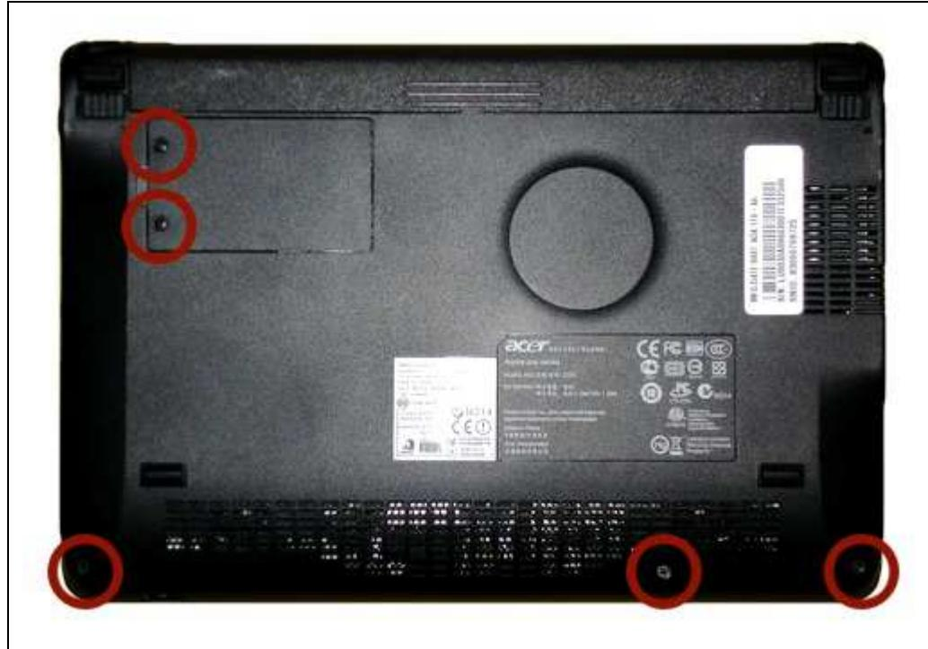
3. Take off the battery and remove the three marked screws.
