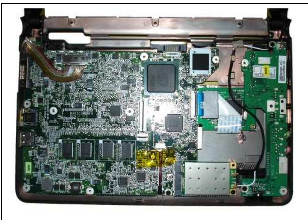
11. Remove the marked screws. The one on the right holds the wireless card in place - once free, the card will spring up and you can slide it out of its slot and move it to the rear of the case.
