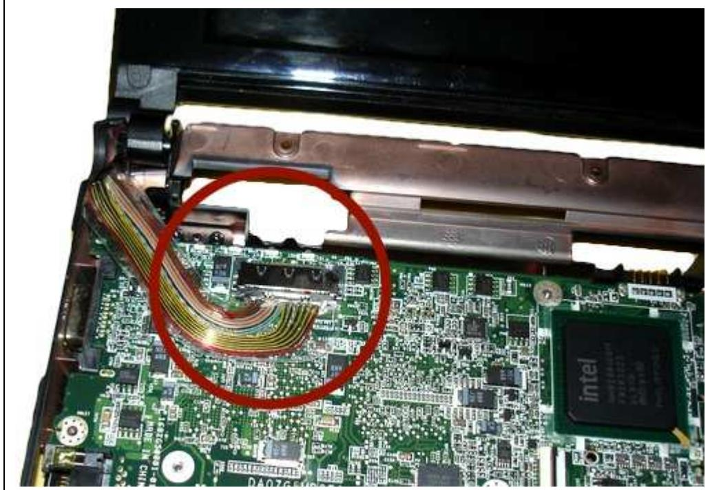
13a. On the right edge of the motherboard, you'll find the SSD connector. It works like the keyboard one: flip up the catch and slip out the cable.
