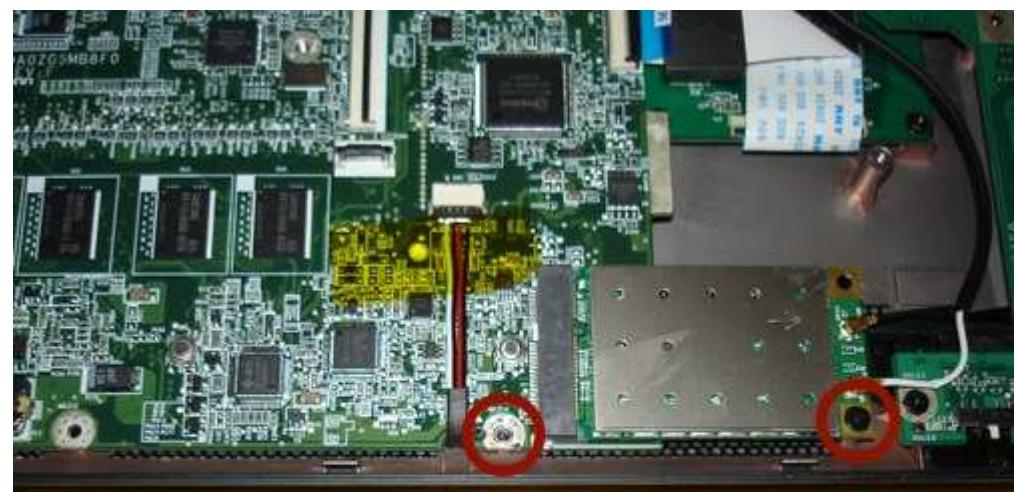
12. Lift the tape holding this cable down - the wires connect the AA1's speakers to the motherboard - and gently pull out the connector. Use the nails on your two index fingers to pull the connector forward and out. Don't just pull the wires.
