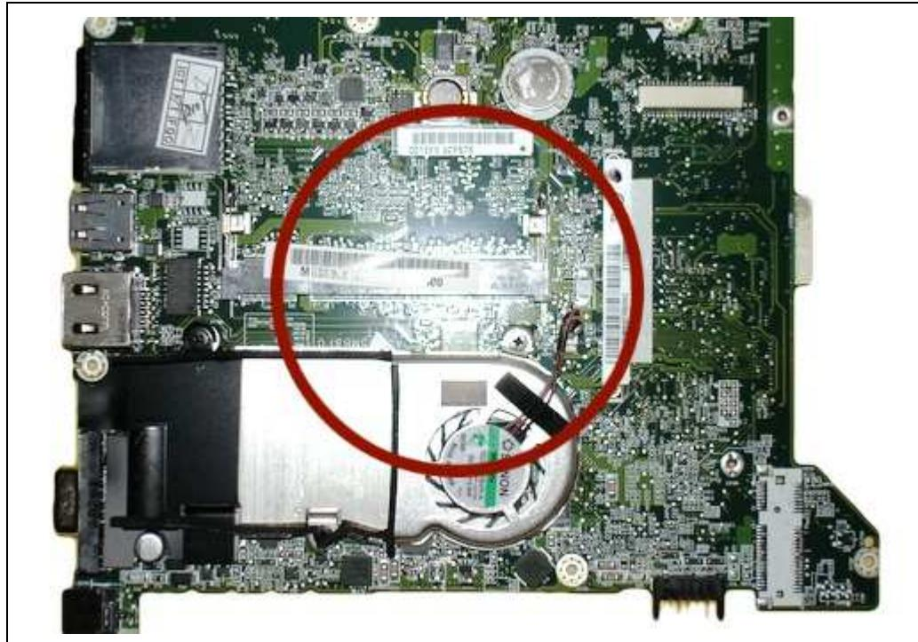
17. ...and clip in your memory card. Use an earthing wriststrap if you have one - if not, touch the bare metal of a nearby radiator pipe to discharge any static electricity on you. When handling the memory, try not to touch the chips and wiring.
