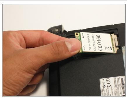
Gently lift the wireless card from its housing starting with the side where the antenna wires were.
