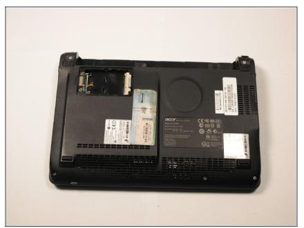
Close display and turn ZG5 over so that the battery compartment is towards the top.
