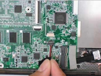
Remove the speaker cable from the motherboard.
