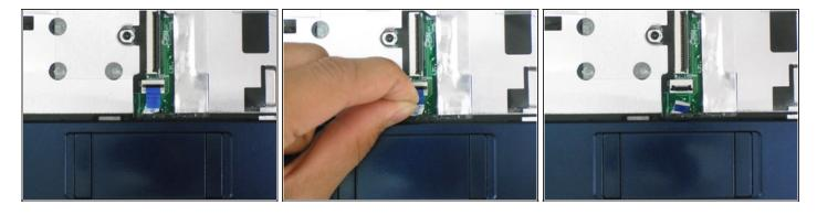
• Gently remove the trackpad cable with the blue tab from the motherboard
