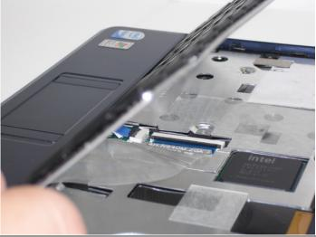
• Lift top of keyboard up. If it doesn't lift easily, there may be tabs on the sides - use the tool to ease them aside and/or shift the keyboard from side to side.
