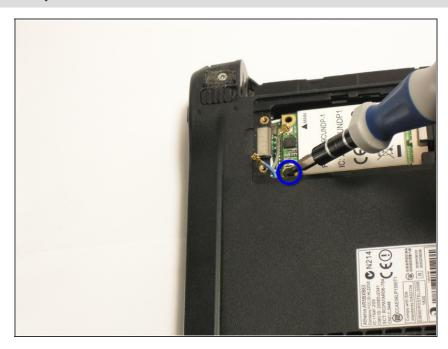
Remove the 3.9mm screw located on the bottom left of the wireless card with Phillips #1 screwdriver.
