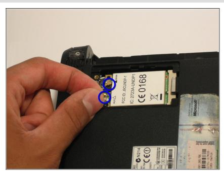
Disconnect the two antenna wires attached to the left side of the wireless card.
